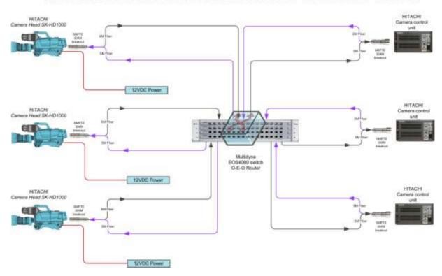
Existing and new fiber infrastructures can be utilized to increase flexibility, offering multiple camera locations all linked via fiber back to the optical routing switcher. The optical router switches the two fibers from each camera and ensures that the SMPTE signal formats are maintained and assigns each camera to the desired CCU.
